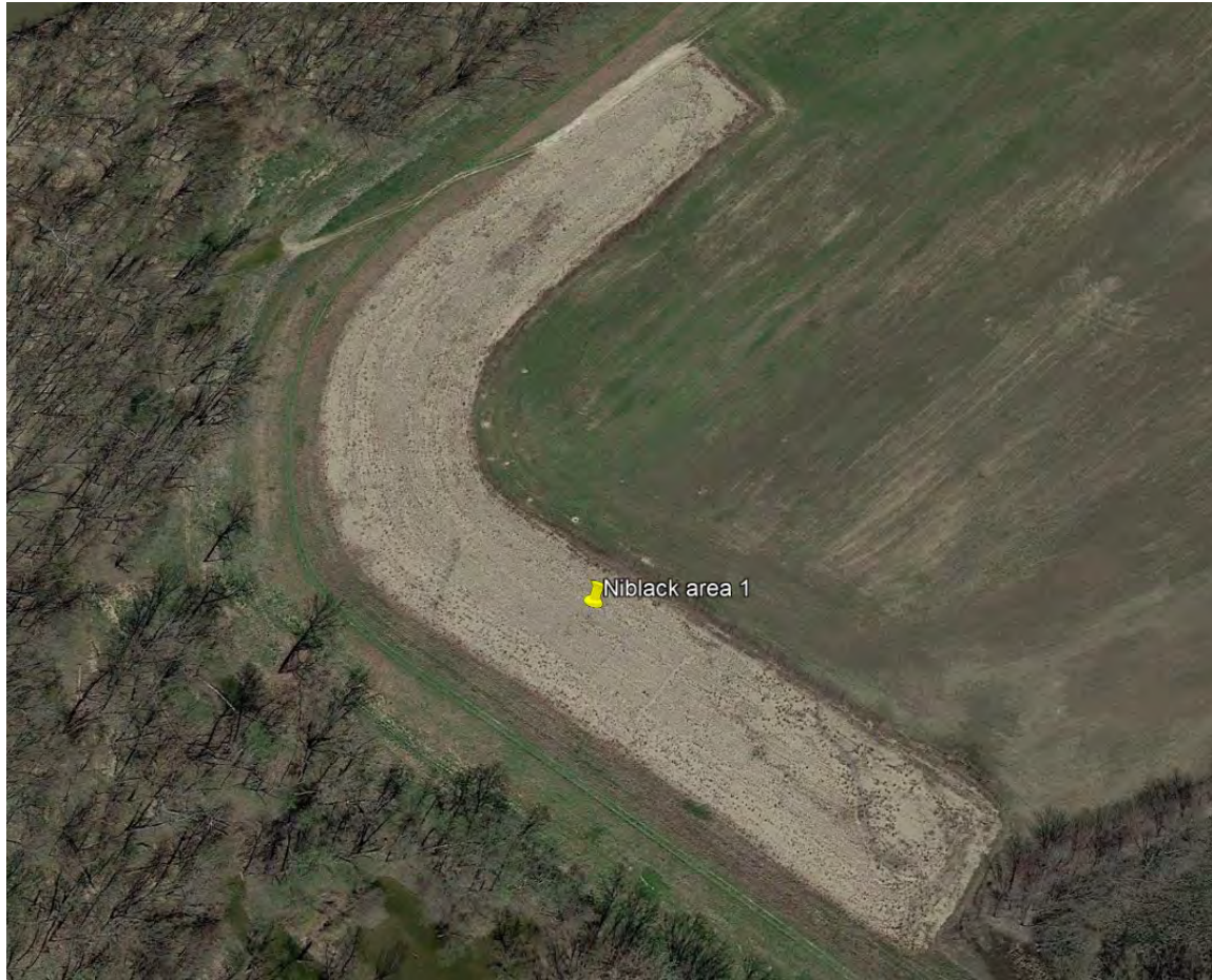
Figure 22. Niblack Sand Berm and Boils Beyond from the 2013 Flood.
