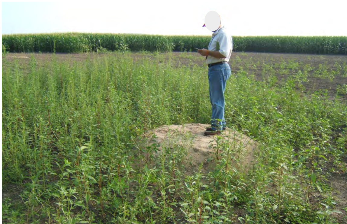
Figure 20. Typical Boil at Niblack 2008
