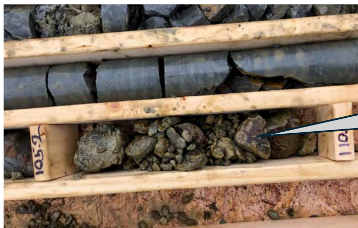
Figure 35 B-5 Shear Zone 105.2-110.2 feet
