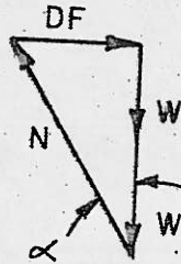
b) POLYGON OF FORCES ASSUMING NO SHEARING RESISTANCE
