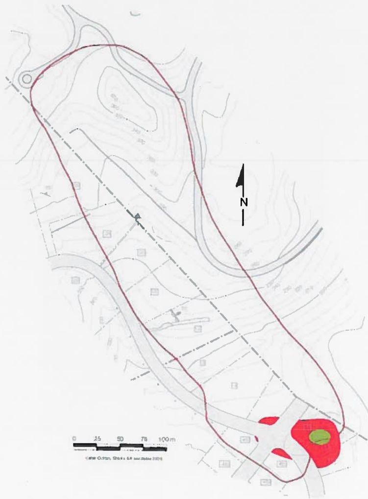
Fig. 4. Plan view illustrating the areas of greater than 3.5 m and 6.1 m (ellipsoidal area) of surface grading
