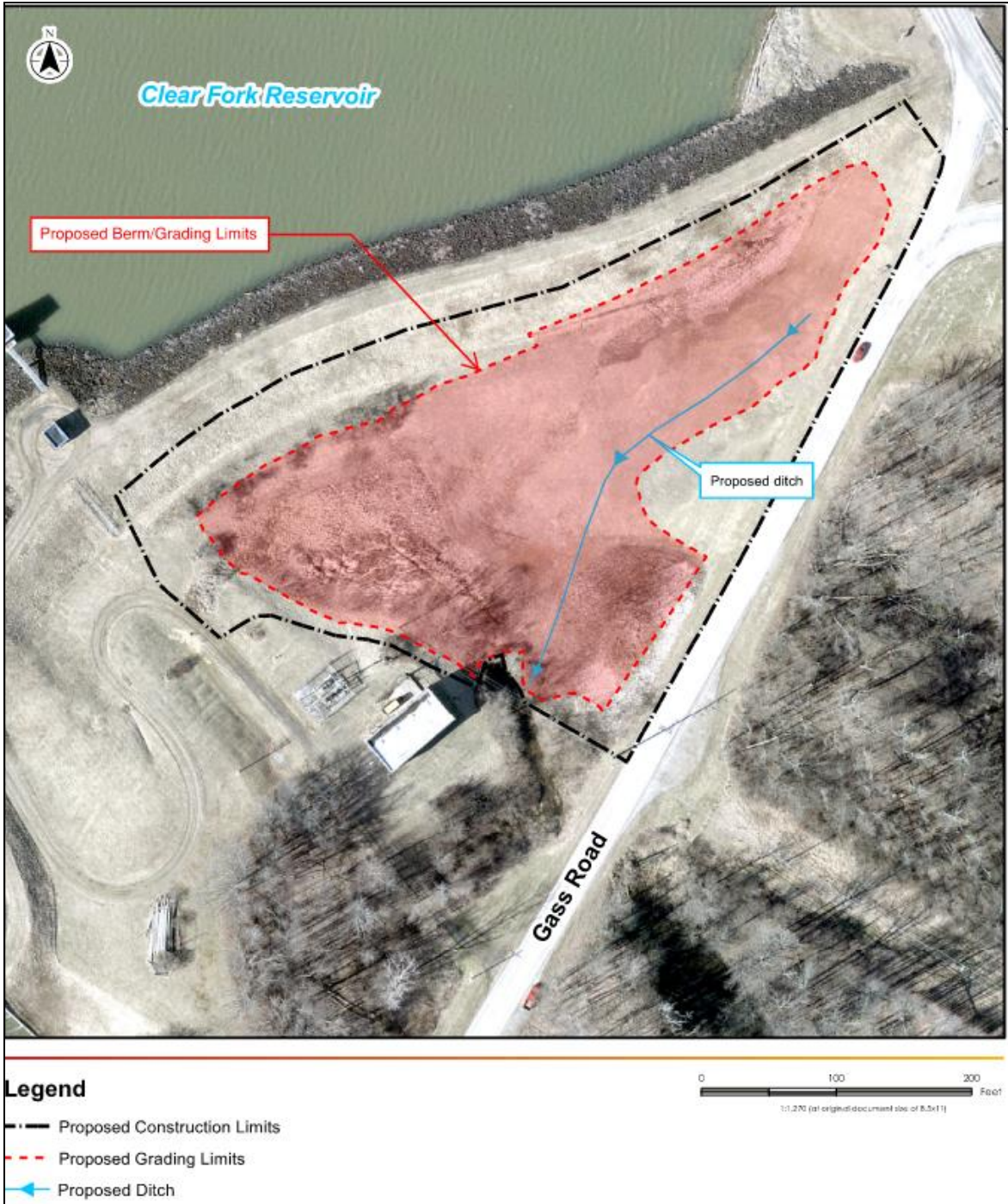
Fig. 11. Graded Filter Toe Berm – Plan View Extents
