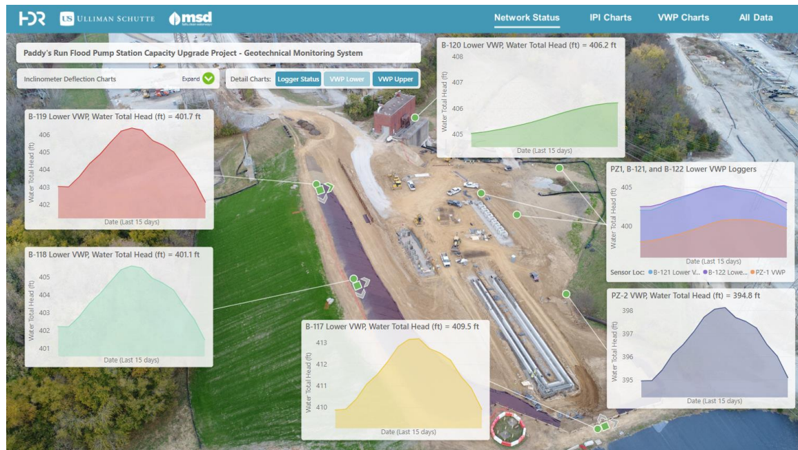
Figure 18: Typical BI Dashboard View of the Monitoring Data Collection
