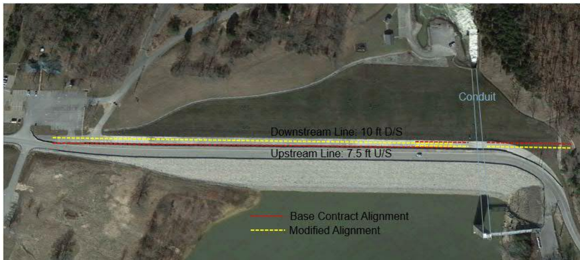
Fig. 10. Rough River Dam Base and Modified Grout Lines
