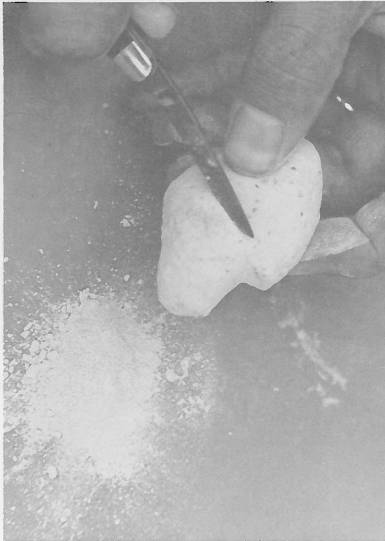
FIGURE 16 SOFT HIGHLY WEATHERED AGGREGATE
